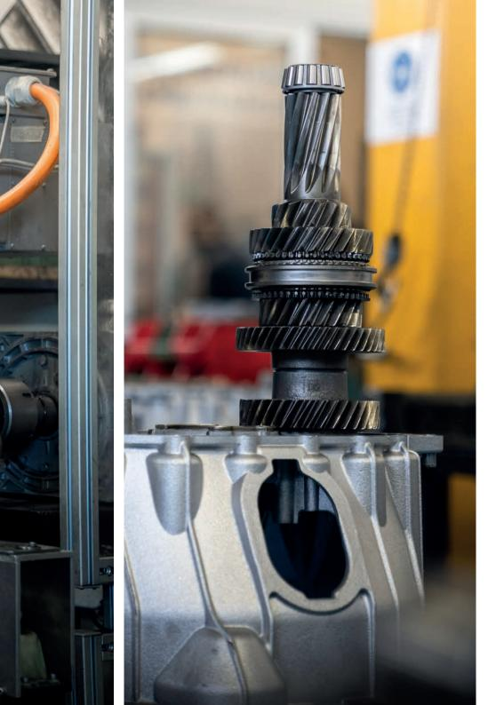
Every remanufactured gearbox is tested with the most upto-date test bench characterized by max efficiency and low noise level.
